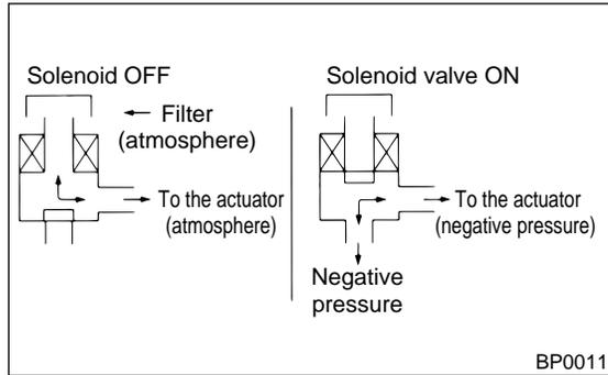
Check if the solenoid valve operates as shown in the illustration above.
