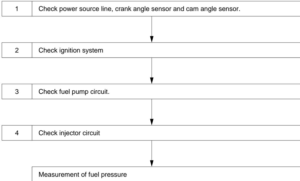
1. Check of power source line, crank angle sensor and cam angle sensor
