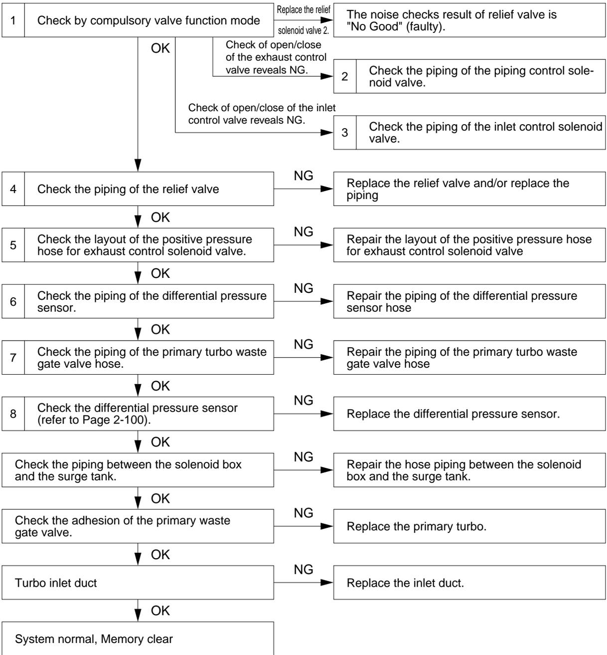
1. Check by compulsory valve function mode
